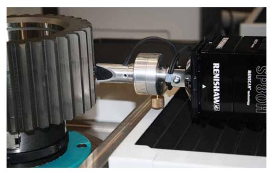
This Wenzel WGT 500 gear measuring machine uses a Barkhausen Noise Analysis system integrated into a horizontally-mounted Renishaw SP80 probe to detect pitting and grinding burn on the ground surfaces of gears.
