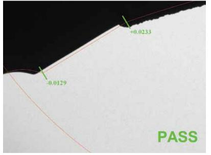
Bidirectional tolerances at various control points can be specified by the user. The system automatically computes and displays the part's deviation from nominal at every control point. This display includes a pass/fail result at every control point as well as for the entire part.
