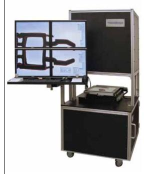
The VisionGauge can be configured either horizontally or vertically, as dictated by fixturing and mounting considerations.
