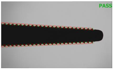
The Tooth Checker tool can check that either crests, roots, or both, are in tolerance
