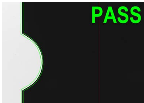
Automatically compare a part to its CAD data and get an accurate, repeatable and operator-independent PASS/FAIL result
