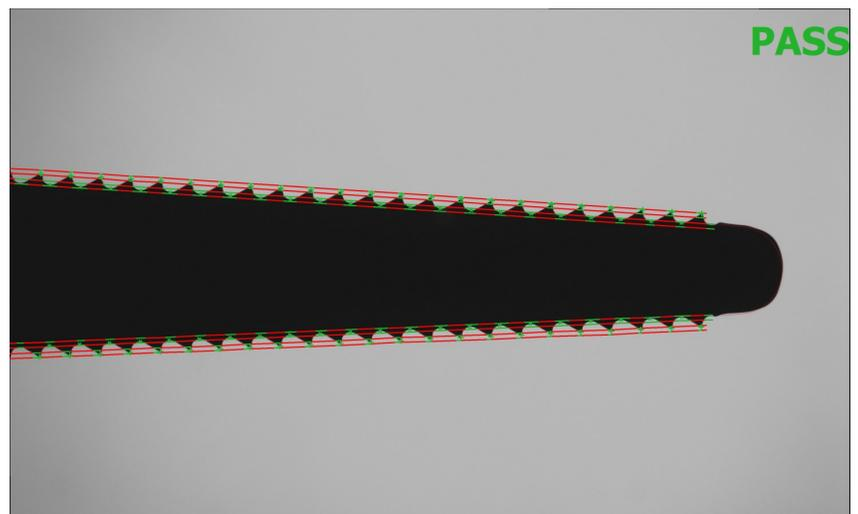
The Tooth Checker tool can check that either crests, roots, or both, are in tolerance
