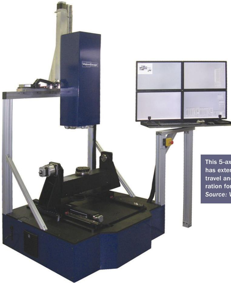
This 5-axis inspection system has extended 24" x 24" x 24" travel and trunnion configuration for big, heavy parts.
