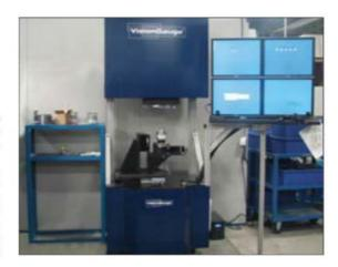
The 700 series has linear axes with 0.25-micron resolution and a 0.005-inch resolution on the rotary axis. For both round and shaped holes, the VisionGauge 700 Series automatically verifies precise hole presence and accurately measures hole location — typically achieving repeatability of ±0.0001 inch.
