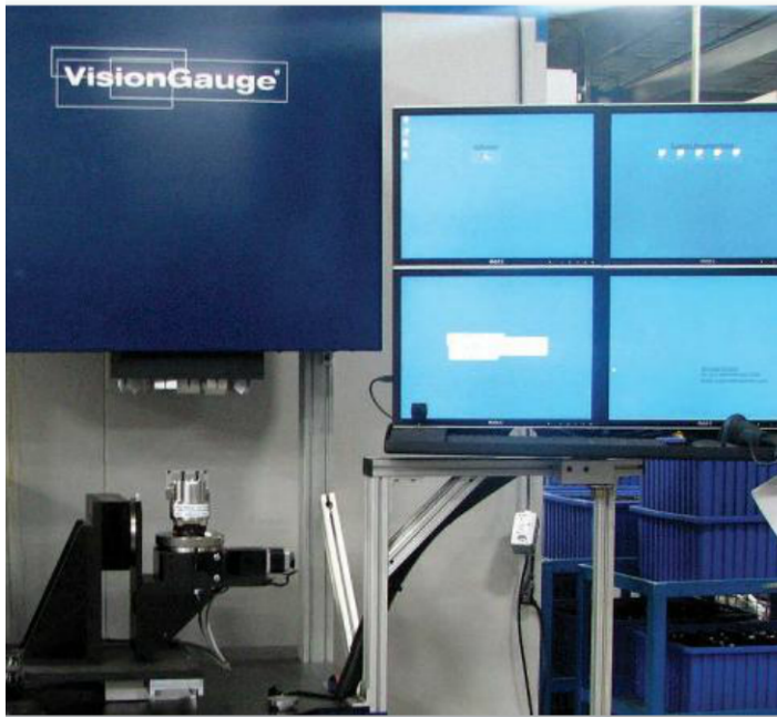
Display monitor shows holes to be inspected on Paradigm Precision's VisionGauge 700 Series Digital Optical Comparator.
