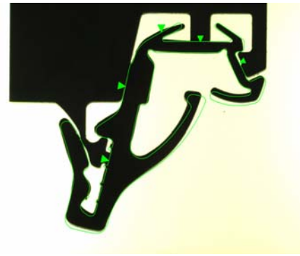
Live Image Overlay Builder with Support for DXF Format CAD Files: Compare your Part to the CAD Drawing
