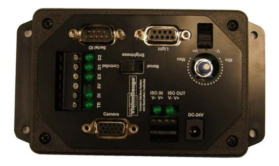
The VisionGauge® Camera Interface Module and Illumination Controller can be used either in conjunction with any of the Sony Smart Cameras or as a "stand alone" illumination controller.
