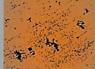
Image 5: Result of thresholding operation after noise reduction and uneven illumination correction
