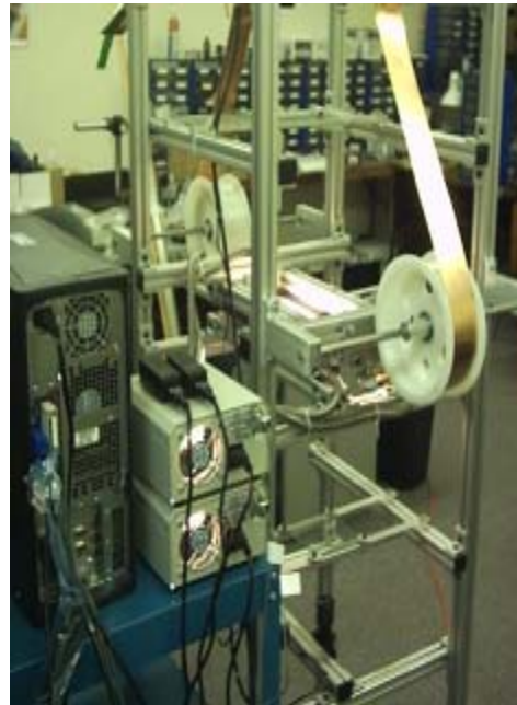
Metal strips are fed through the inspection Area where dual cameras capture computer controlled illuminated images of the strip for processing.
