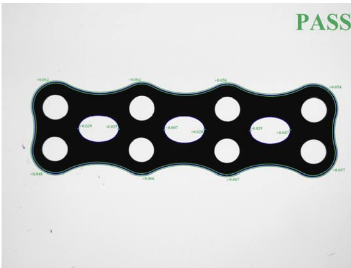
Patented VisionGauge® CAD Auto-Align™ and CAD Auto-Pass/Fail™ tools provide fast, accurate and operator-independent results
