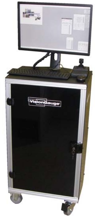
Remote cabinet with controls, user interface & I/O connections
