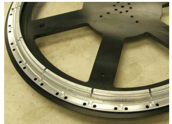
Ring with cooling holes. For larger rings, it is typical to use an extended-travel 700 series system to check the hole presence and measure the hole location & geometry
