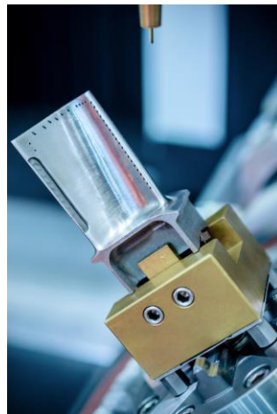
5 Axes of motion to properly view part from all sides & angles
