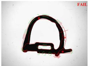
Automatically compare a part to its CAD data and get an accurate, repeatable and operator-independent PASS/FAIL result
