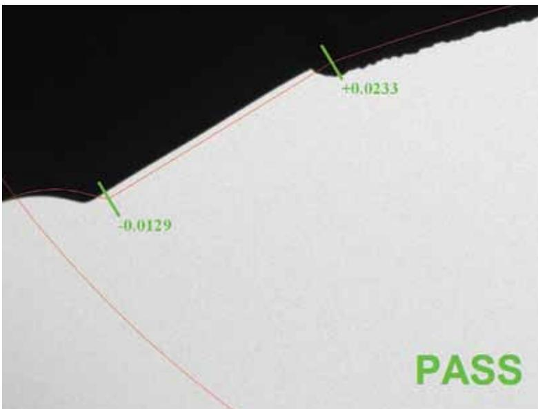
Bidirectional tolerances at various control points can be specified by the user. The system automatically computes and displays the part’s deviation from nominal at every control point. This display includes a pass/fail result at every control point as well as for the entire part.
