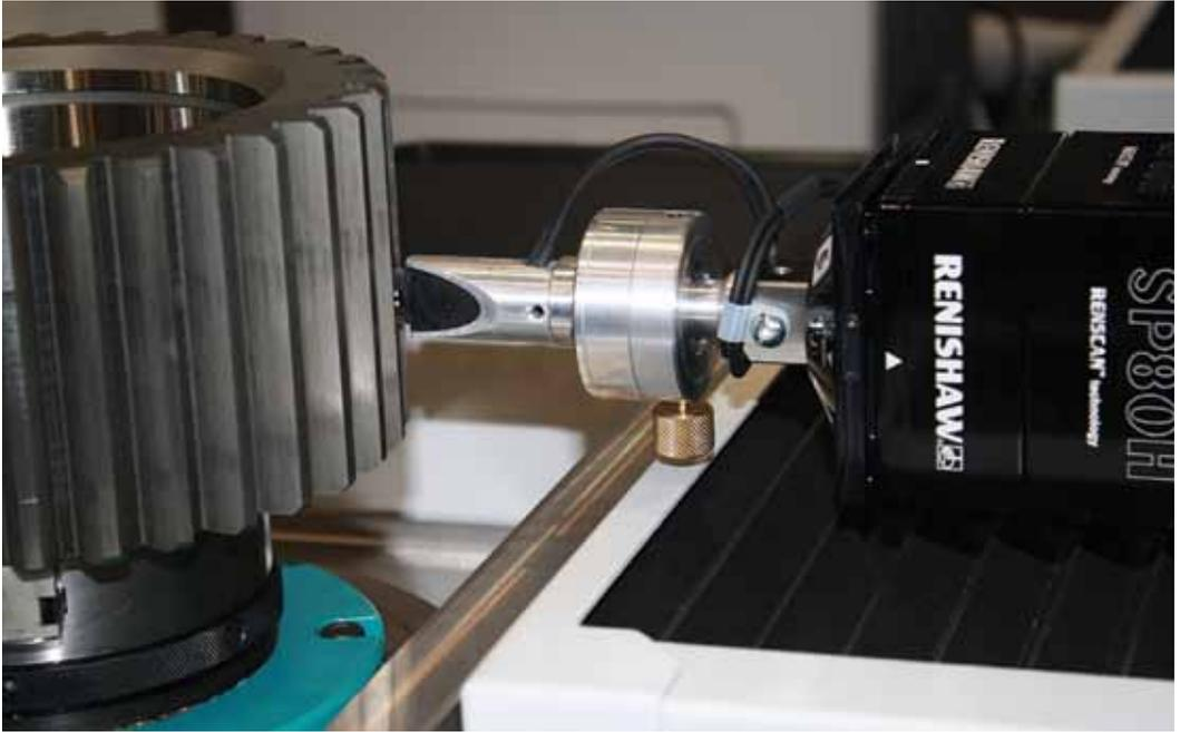
This Wenzel WGT 500 gear measuring machine uses a Barkhausen Noise Analysis system integrated into a horizontally-mounted Renishaw SP80 probe to detect pitting and grinding burn on the ground surfaces of gears.
