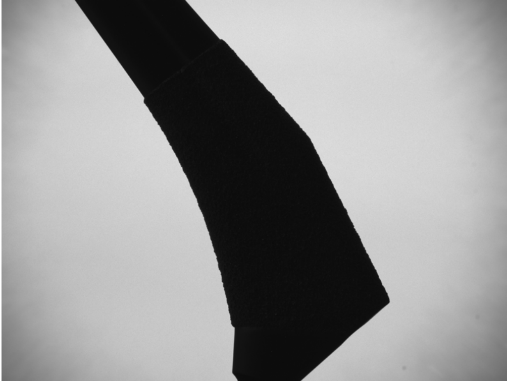
Image of a part (an orthopedic hip implant) using traditional transmitted (i.e. back) illumination. This produces the maximum edge / profile sharpness.
