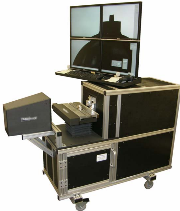
Overall view of the VisionGauge® Digital Optical Comparator. In this picture, we can see the collimated LED back illumination module (on the left), the stage and column (towards the middle of the picture) and the quad monitor display (top).
