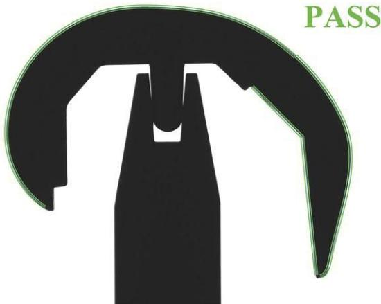
In this image, the system is automatically comparing the condyle (part of a complete knee replacement system) to its CAD data. Source: VISIONx
