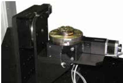
The 700 Series VisionGauge digital optical comparator features a chuck mounted on its double-rotary assembly.
