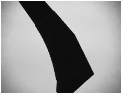
Image of a part using traditional transmitted (i.e. back) illumination. This produces the maximum edge / profile sharpness.
